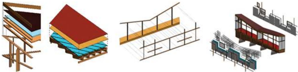
Fig. 8. Exploded views of the 3D model used to visualize building assemblies and the interplay between building components and materials. Image edited by the authors.
