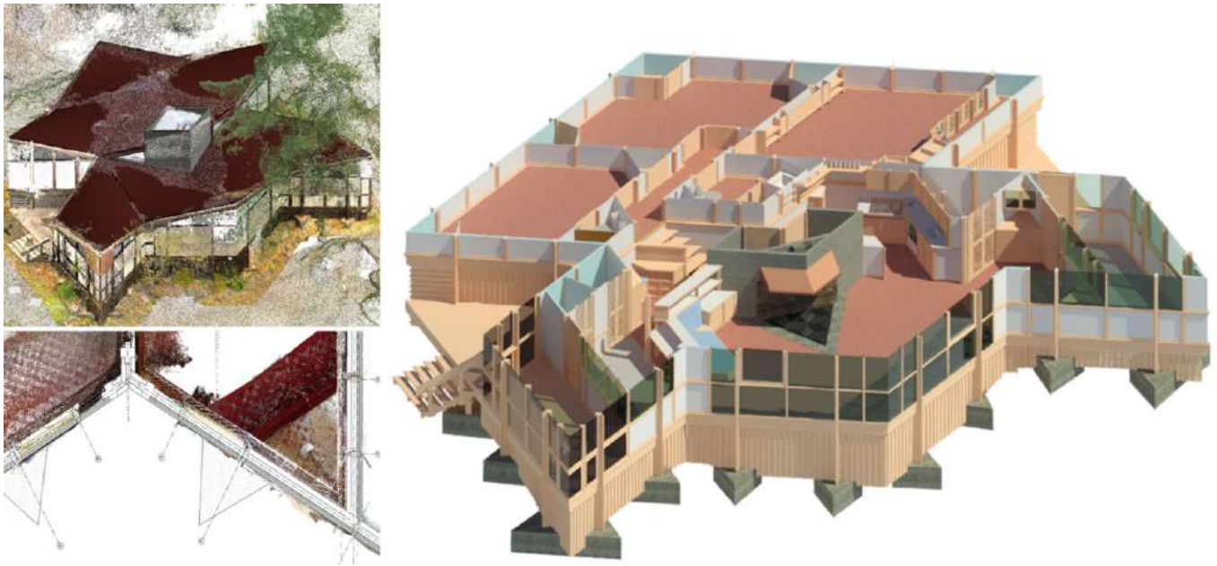
Fig. 7. This image illustrates the modeling workflow with the mapping of parametric objects onto the point cloud and the superposition of the point cloud with the HBIM model of the house (left); an overview of the final model with a section perspective showing the lower and upper level of the house (right). Image source: authors.
